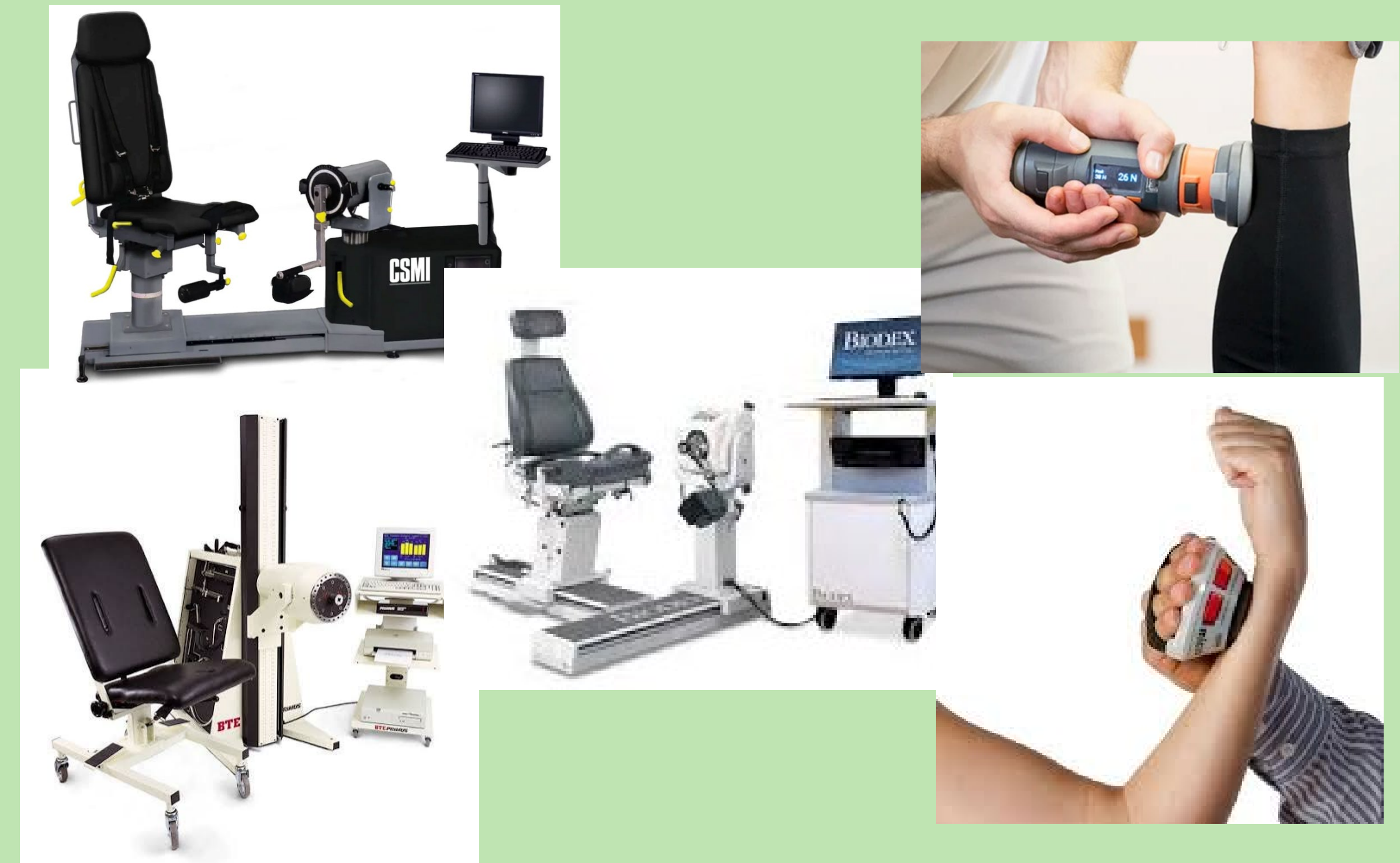
Figure 1: On-Market Isokinetic / Isometric Muscle Measurement Devices. A variety of current options for measuring muscle force / torque. Footprints of the devices vary from small to large. Some devices require practitioner-dependent counterforce. (From left to right: HumacNORM , VALD DynaMo , BTE Primus RS , Biodex 3 , MicroFET2 ).
