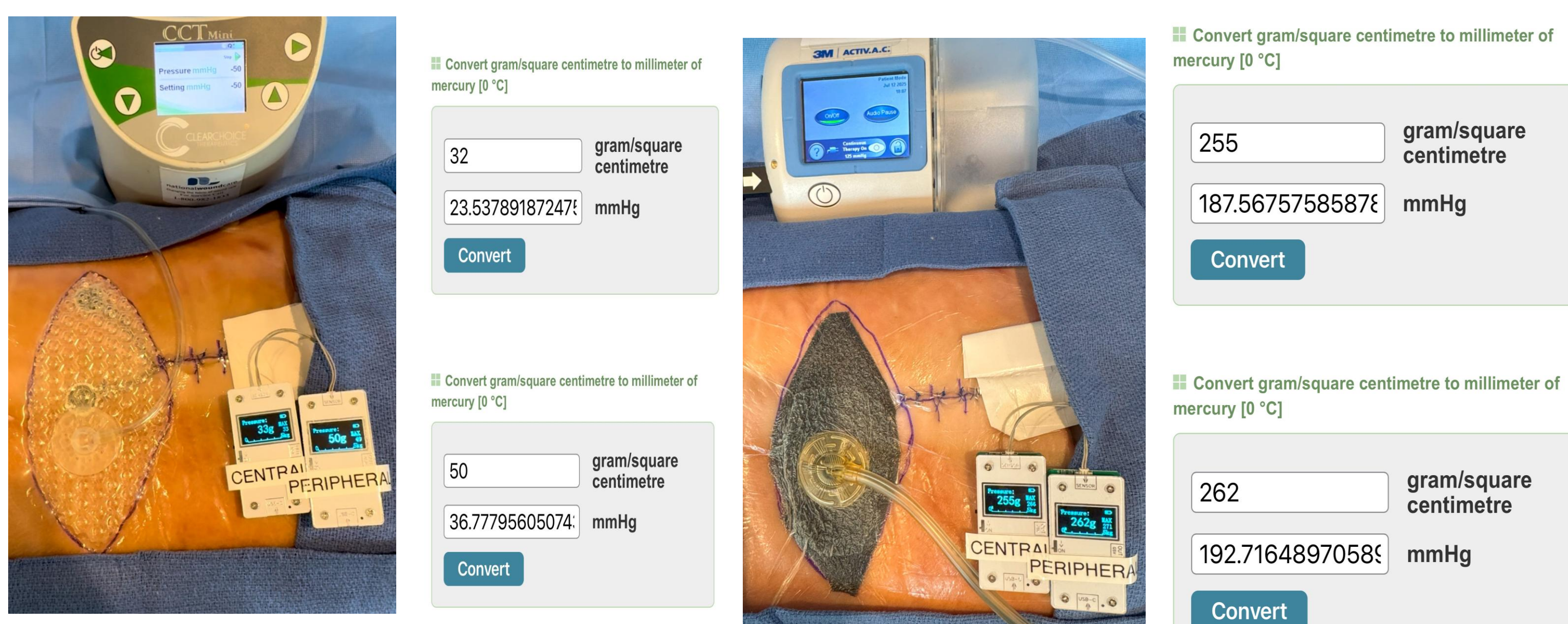
Figure 3: Images of the TPE at -50mmHg and foam at -125mmHg. Conversion from g/cm 2 (on screen) to mmHg shown to the right
