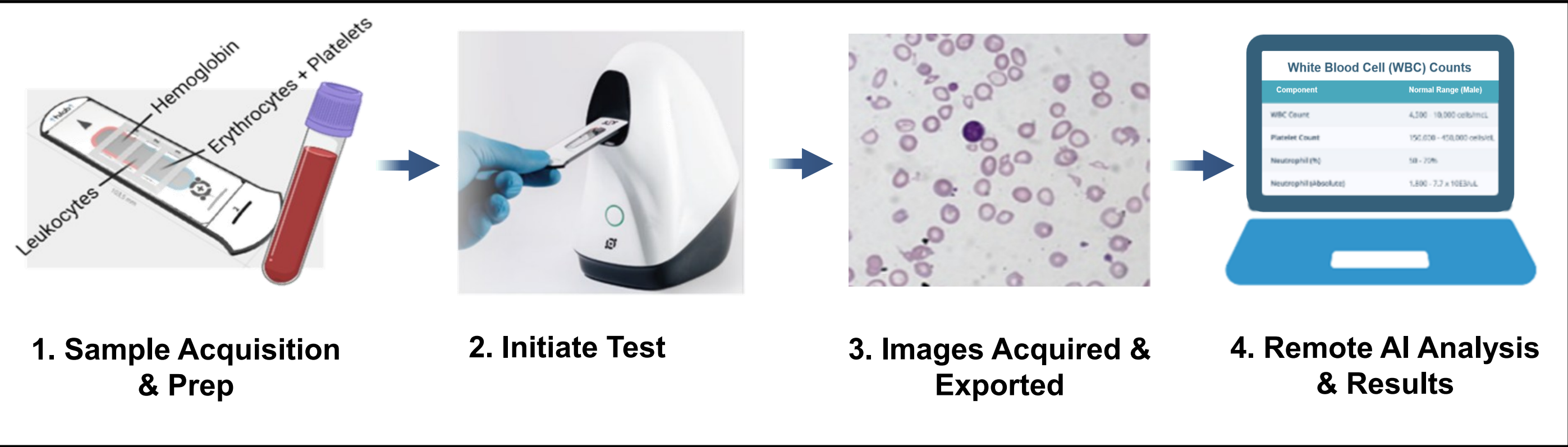
Figure 2. Schematic of Lens sample processing
