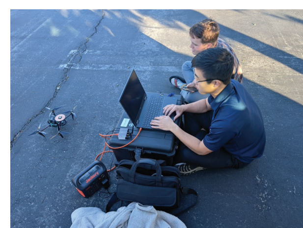
Ground Station: Drones sends images and GPS back to station and RL agents send control commands
