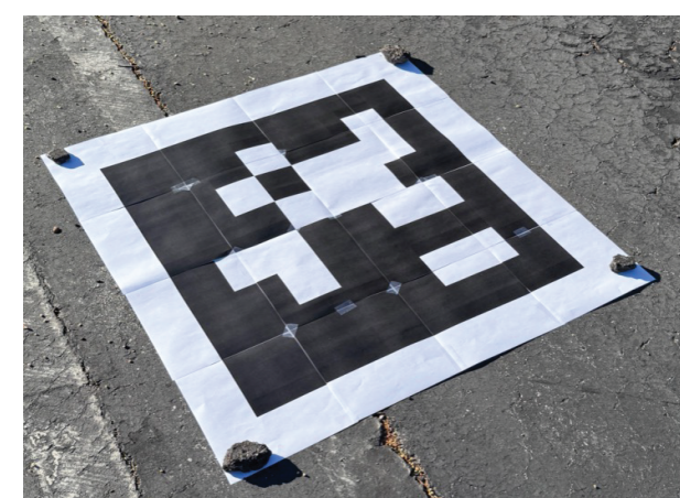
April Tag: Used in place of casualty dummies, each tag encodes a different injury severity value
