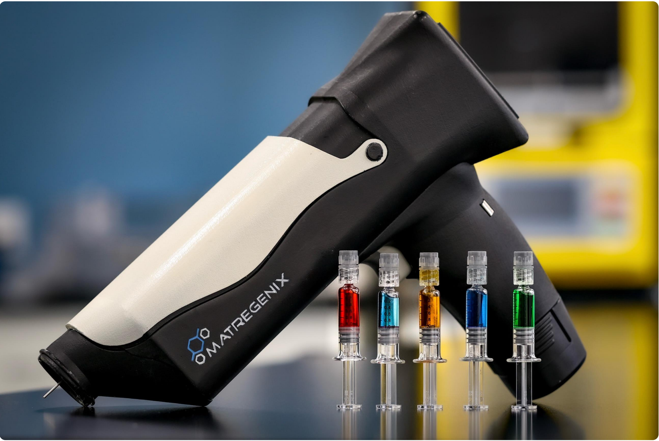
Portable investigational electrospinning system for in-situ deposition of a conformal nanofibrous primary wound dressing.
