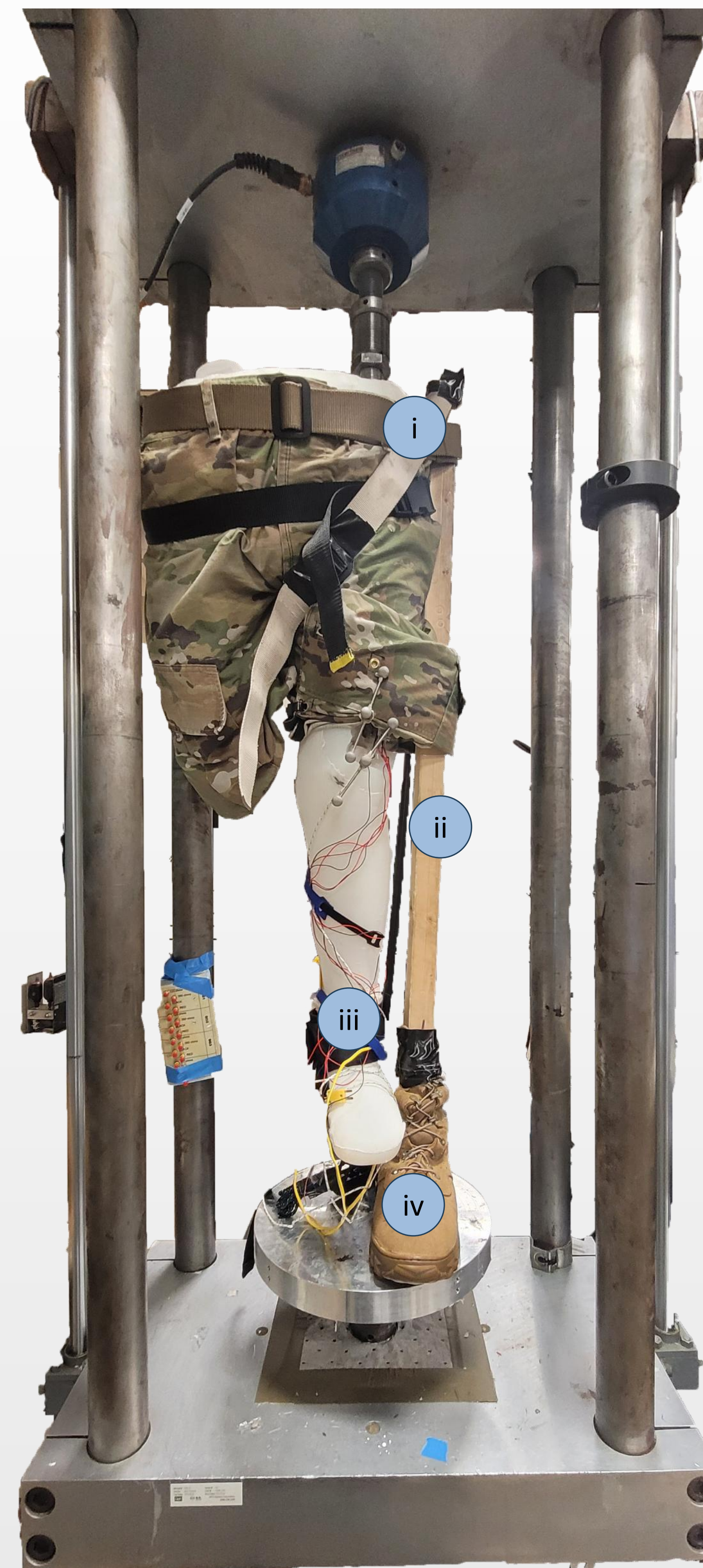
Figure 1: Lower extremity design for a LE fracture in a MTM highlighting 4 distinct components: i) Suspension, ii) Support, iii) Splint, and iv) End effector. Components were constructed from different materials listed below.
