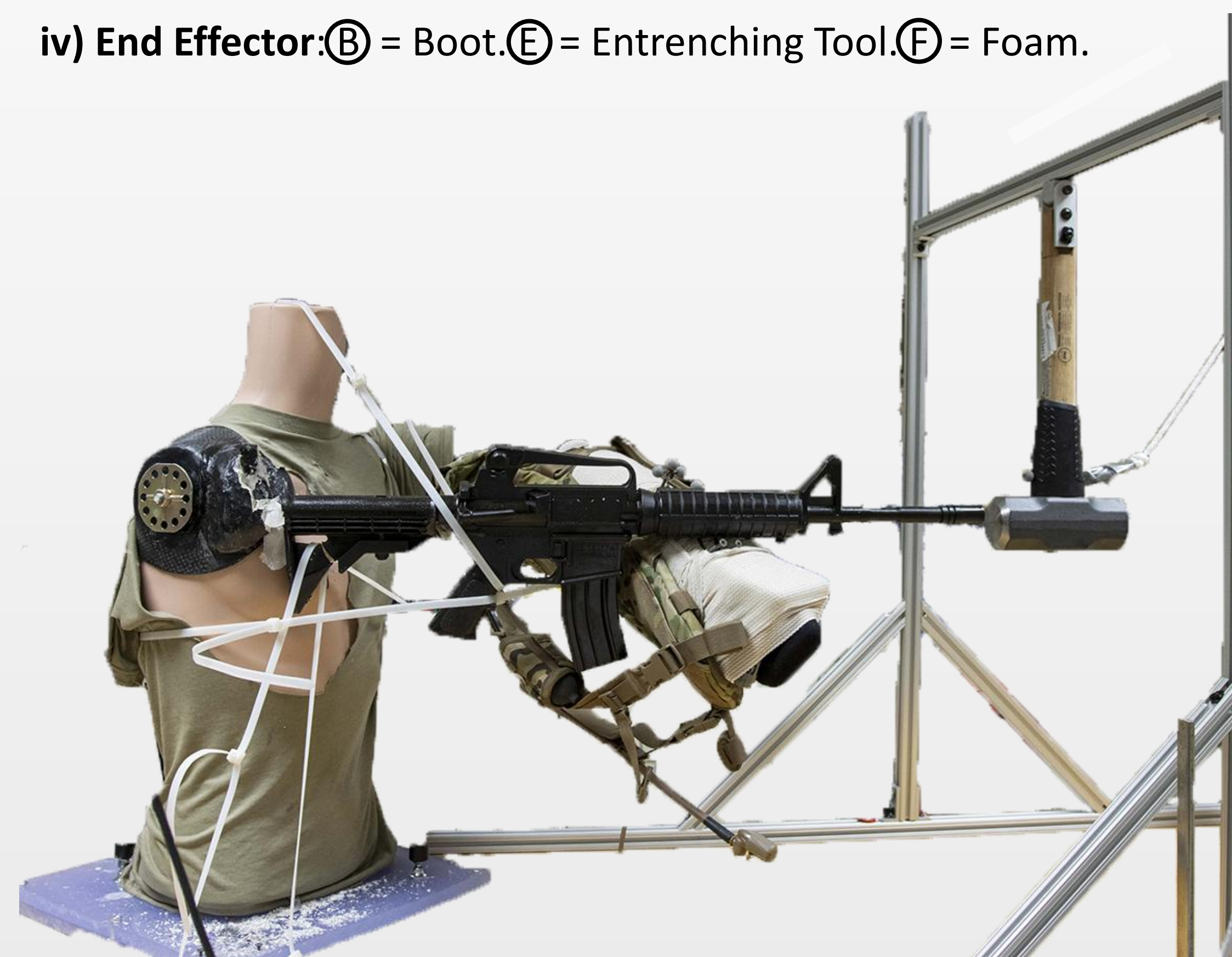
Figure 2: Upper extremity design for a radial/ulnar fracture being tested with a ballistic pendulum.
