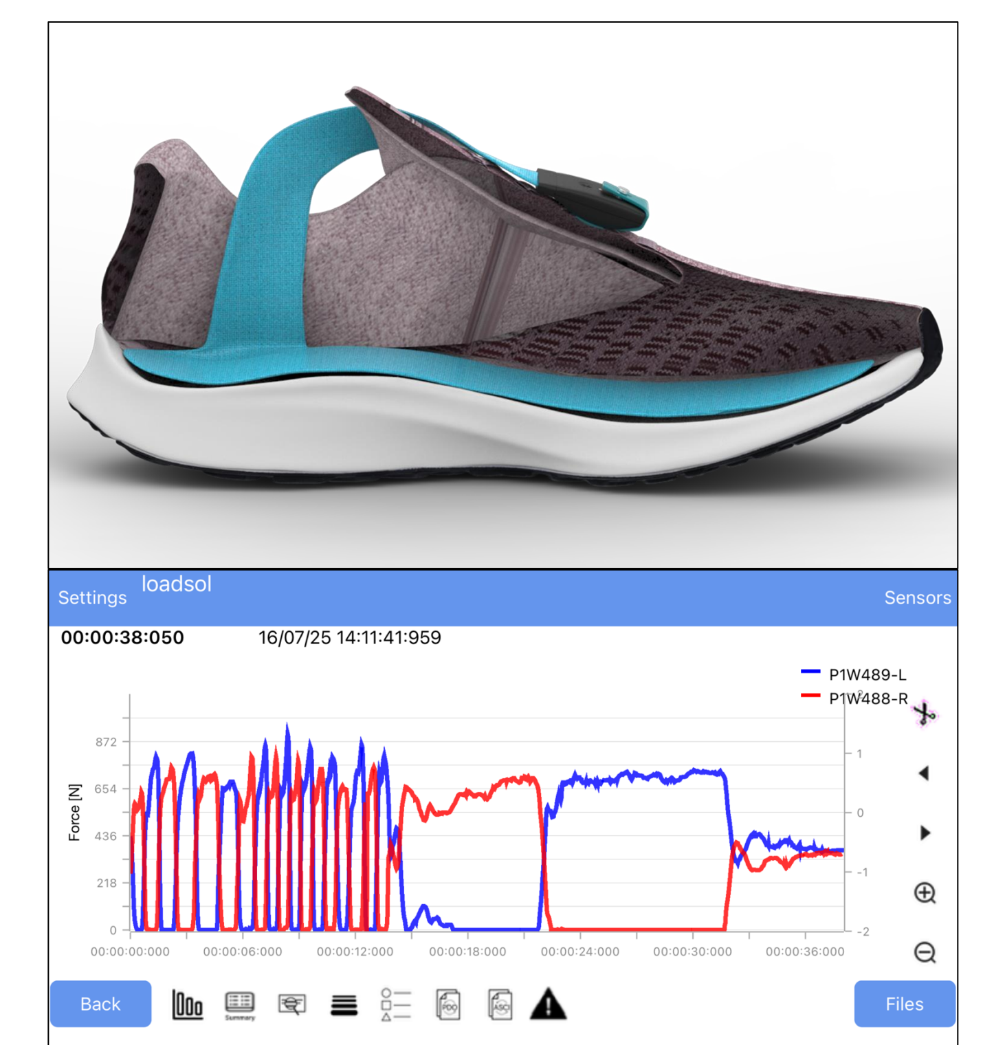
Figure 2. Instrumented shoe insole (top) and iOS app used for biofeedback training (bottom)
