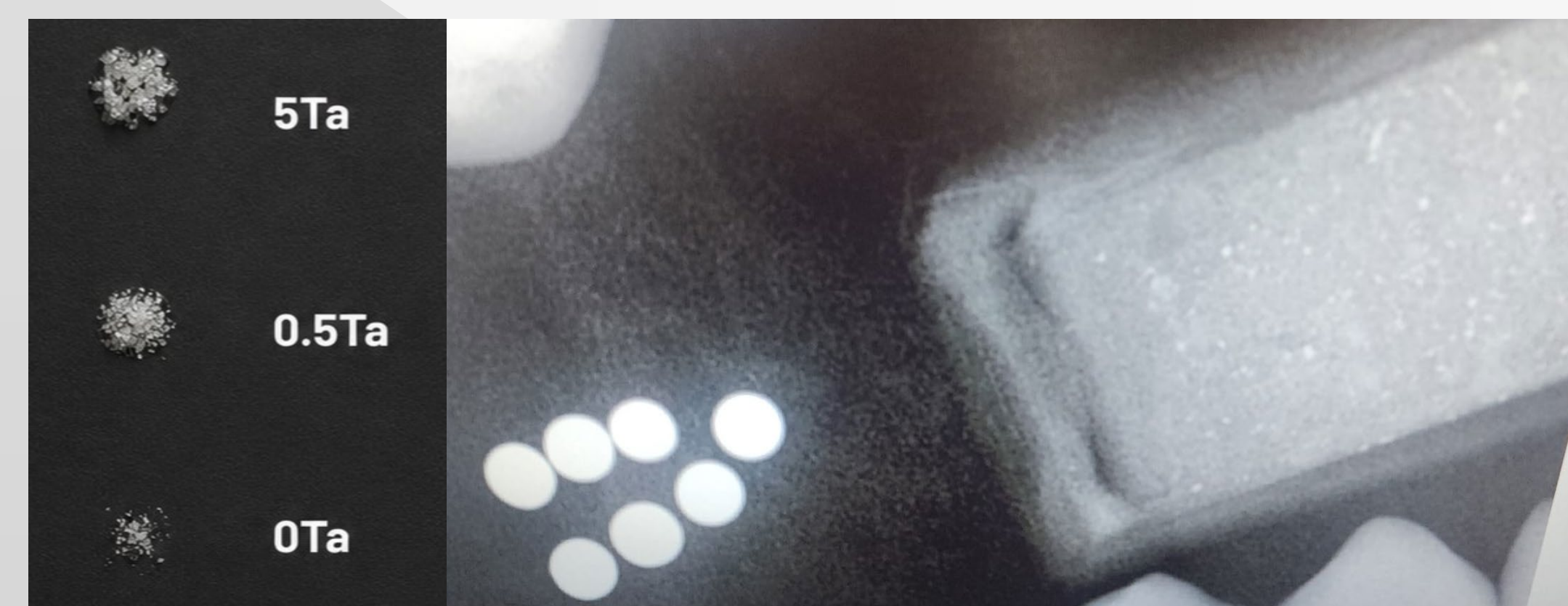
Figure 3 (Above). Radiopacity of Ta-MBG (Left: DEXA of 0, 0.5 and 5 mol Ta-MBG) Right (Intraoral X-ray of 5%Ta-MBG powder with Pb shots as reference)
