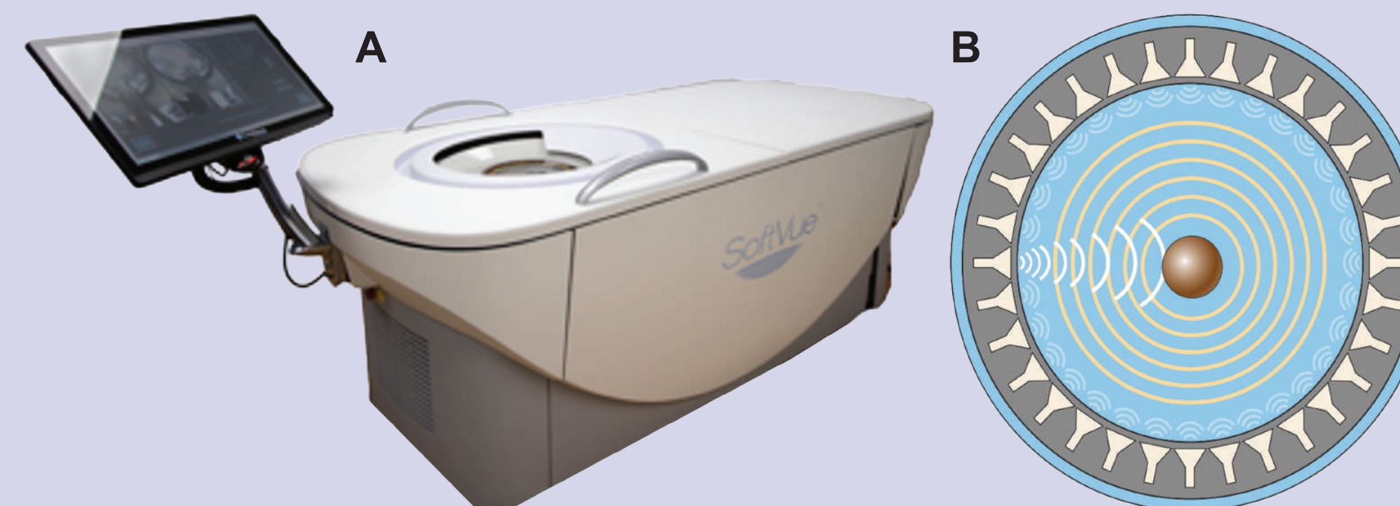
Figure 1. A) The SoftVue clinical UST imaging system. B) Overview of the UST synthetic aperture data acquisition. The system transmits on one element at a time and receives on all 1024 elements before advancing to the next transmit element.
