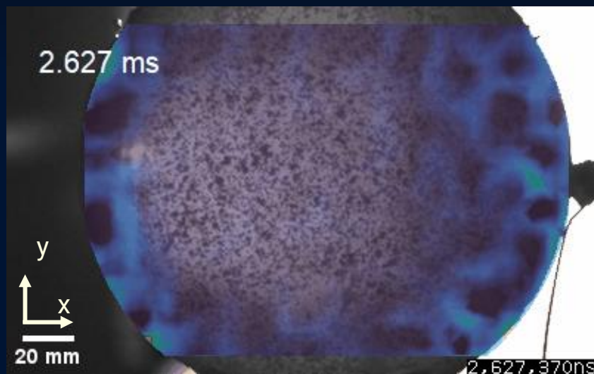
Shock front tracking via DIC (BOP: ~16 psi)
